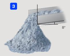
With fluidization, gravity flow can be achieved at a greatly reduced slope - of  $8^{\circ}$  or less.
