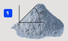
All dry bulk material has a natural angle of repose, often in excess of 45°.
