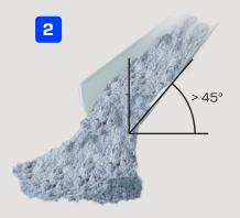
Without any fluidization, the Airslide® conveyor would need to be inclined on an angle greater than the angle of repose to establish gravity flow.
