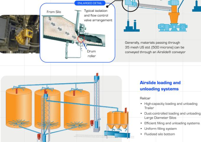
FLSmidth's Airlift™ vertical conveyors and Airslide® gravity conveying systems convey alumina at a net rate of 750 mtph in a major western United States facility
